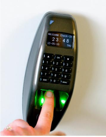
Figure 2 A fingerprint reader with a keypad for a PIN
