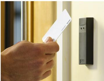
Figure 1: A token in use with a reader working on a proximity basis
